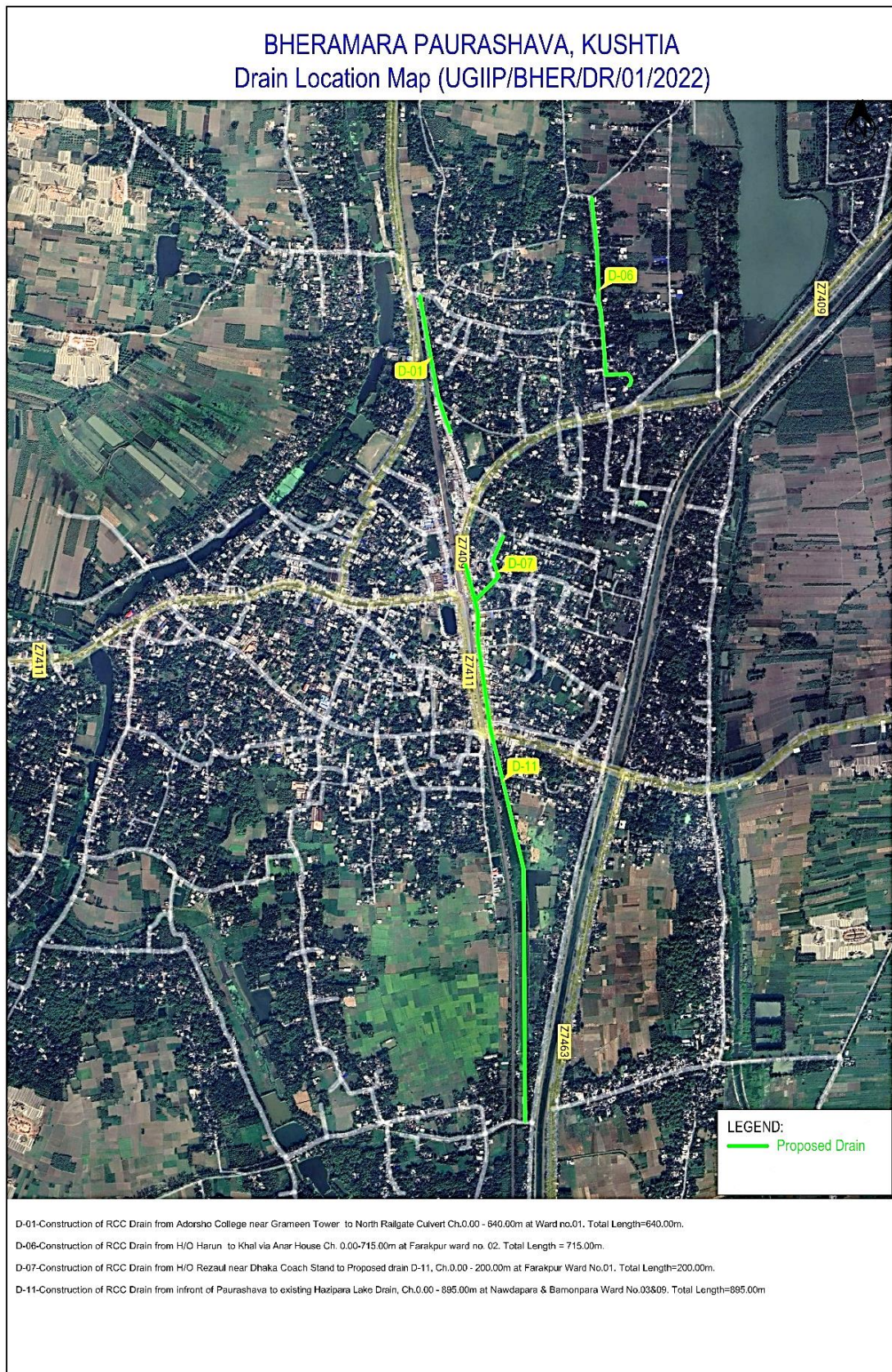
Figure-4: Four Drains Location in Bheramara Paurashava
